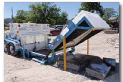
Figure 17. Delivering hardened concrete to a recycler
