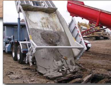
Figure 15. Delivering hardened concrete to a recycler
